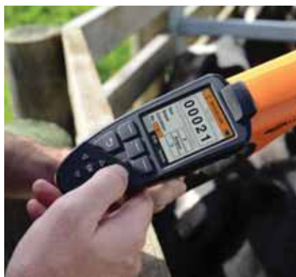
Use pre-defined 'lists' with the HR4 to record traits such as breed or sex and sort into colour coded draft groups.
