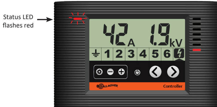
Controller showing the energizer in output alarm
