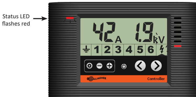
Controller showing the energizer in current alarm
