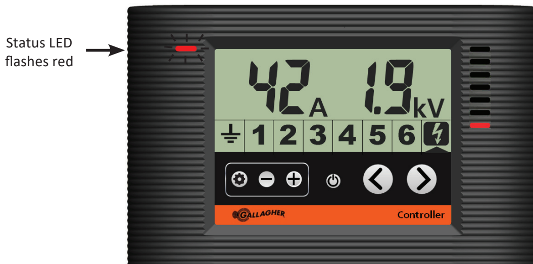
Controller showing the energizer in output alarm
