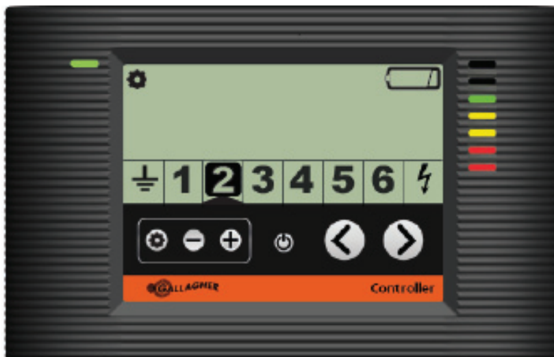
Controller showing zone 2 with a low battery
