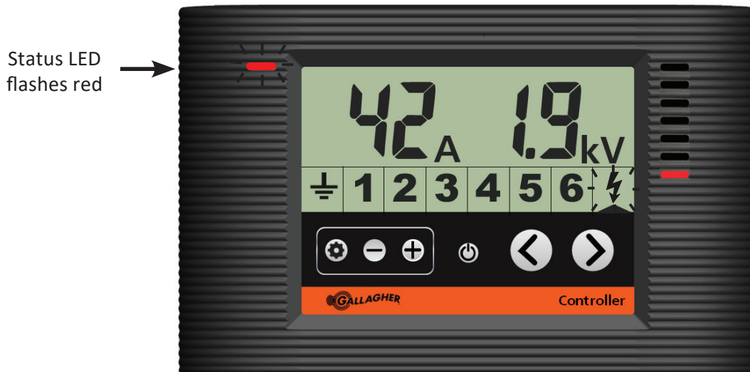
Controller showing the energizer in current alarm
