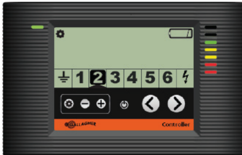
Controller showing zone 2 with a low battery
