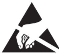
**ATTENTION:** This equipment contains components that can be damaged by electrostatic discharge. Ensure both you and the equipment are earthed before replacing the battery.
